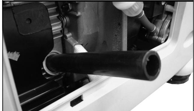
4. Tilt the generator to allow the oil to drain out of the oil reservoir into a suitable container.
