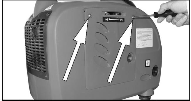
2. Remove the three air filter cover screws .
